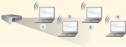
Secure wireless projection with WEP 64/128-bit and session login security protection to prevent unauthorised access to information on the wireless transmission.
