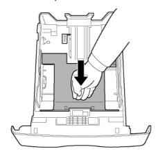
3 Setup the back side feed cassette stop by pushing the "PUSH" lever (A).
