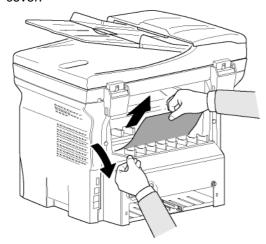
3 Open and close the Front cover. The printer starts again automatically.
