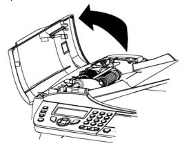
3 Clean the rollers of the document feeder and the two idler rollers located on the mobile part of the scanner with a soft lint-free cloth dampened with mild alcohol.
