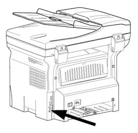
2 Connect the power cord to the device.
