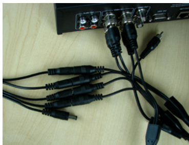
Example of a DVR with camera cables plugged in
