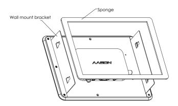
**Step 2**: Remove the six screws (three on each side) at the back and place the wallmount brackets onto the display. Secure the brackets with the original six screws.
