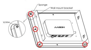
**Step 4**: Insert the display to the surface (opening) where you are going to mount the display
