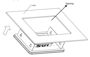
**Step 5**: Attach the mounting clips to the four fillisters on the wallmount brackets and tighten the four M4x60 screws to secure the brackets
