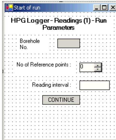
This screen is used to set up the number of reference (zero correction) points and the interval (distance) between readings. It will default to the first profile in the list, but this can be changed by selecting the appropriate one from the drop-down list. If this is done, when the screen is completed and the user is taken through to User Screen 2, the selected profile will be remembered.
