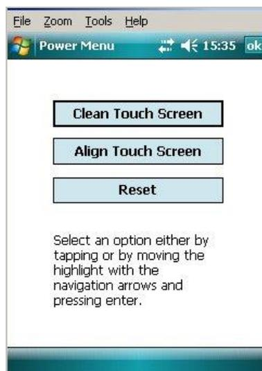
Tapping "Reset" will start a reboot of the Field PC, closing any running programs without losing any installed programs or settings.
