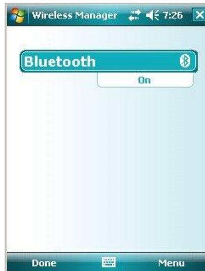
Tap on the Bluetooth icon on the main screen, a "Bluetooth bar" will appear, tap on this bar to set Bluetooth to "on".
