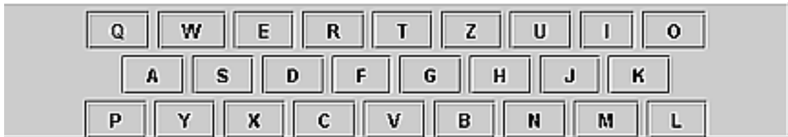
Figure 16. Keyboard Panel, made up of three tiers of JPanels, each tier using a flow layout
