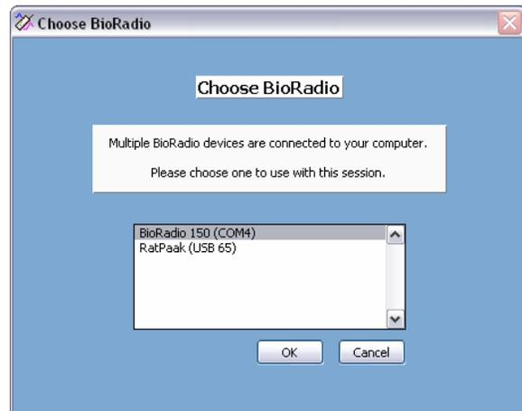
A *Legacy Device* is connected to the PC, using USB, identically as a non-legacy device, but recognized as USB→Serial interface and communicated with through a serial COM port. Currently, the RatPaak is the only BioRadio device with non-legacy support, acting in a "purely" USB manner.
