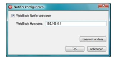
**Activate WebBlock Notifier** Aktivate the WebBlock Notifier and enter the computer name or IP-address of the computer on which the WebBlock 2011 Software runs (usually the server/main computer of your network).
