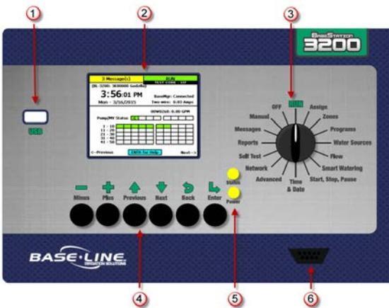
**(1) USB Port** – The USB port is used for doing Backup and Restore operations using a USB drive (also known as a “thumb drive” or a “flash drive”). The USB port is also used for doing firmware updates and exporting operation log files.
