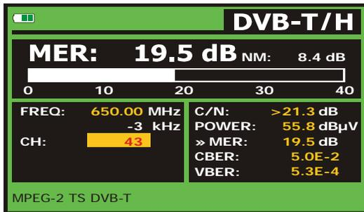
Figure 39.- DVB-T/H (COFDM) signals MER measurement screen.
