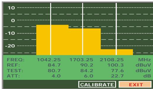
Figure 17.- Attenuation measurements in an outlet plate.
