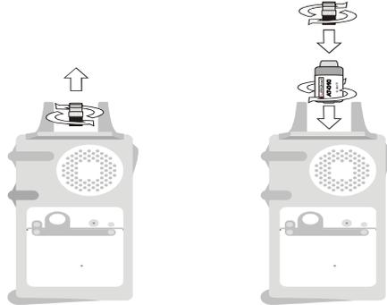
Figure 6.- Connecting external attenuator on RF input [30].
