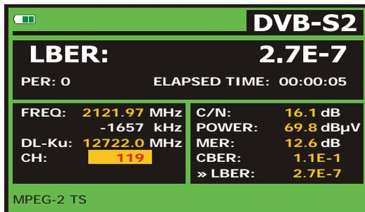
Figure 38.- DVB-S2 (QPSK/8PSK) signals **LBER** measurement screen.
