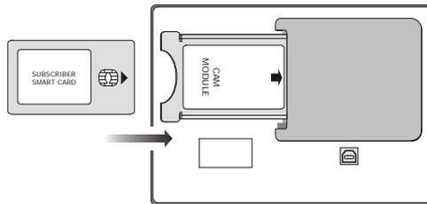
**Figure 62.-** Subscriber Smart-Card and CAM module insertion.
