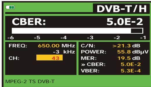
Figure 31.- DVB-T/H (COFDM) signals CBER measurement screen.
