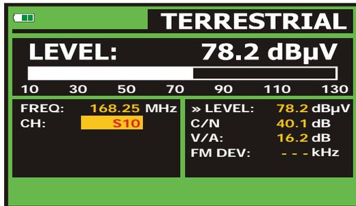
**Figure 22.-** Analogue signal level measurement in terrestrial band.
