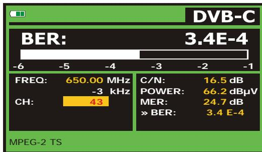
Figure 29.- DVB-C (QAM) signals BER measurement screen.
