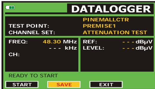
Figure 14.- Datalogger screen for Attenuation test frequencies.
