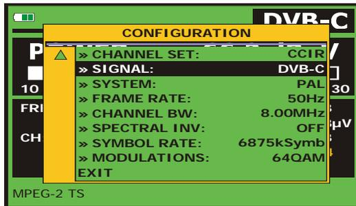
Figure 19.- Screen of measurement configuration (QAM signals).
