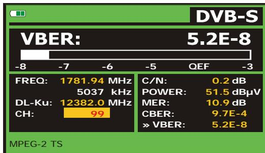
Figure 36.- DVB-S (QPSK) signals VBER measurement screen.
