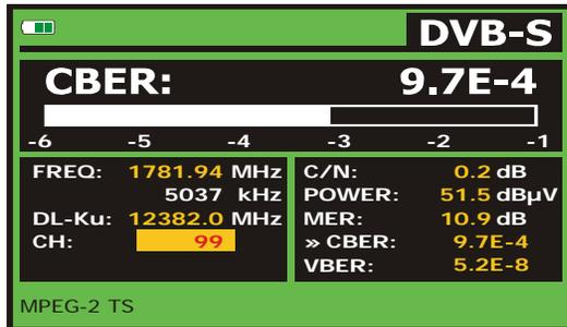
Figure 34.- DVB-S (QPSK) signals CBER measurement screen.
