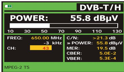
Figure 28.- Digital channel power measurement.
