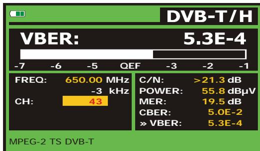
Figure 33.- DVB-T/H (COFDM) signals VBER measurement screen.
