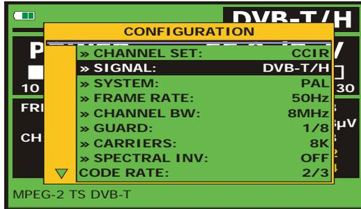
Figure 20.- Screen of measurement configuration (COFDM signals).
