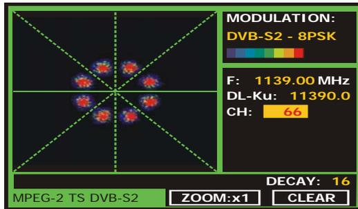
Figure 44.- Constellation Diagram. DVB-S2 (8PSK) signal.
