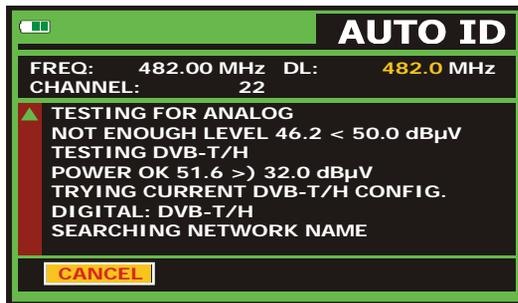
Figure 9.- Signal automatic identification screen. **AUTO ID**.
