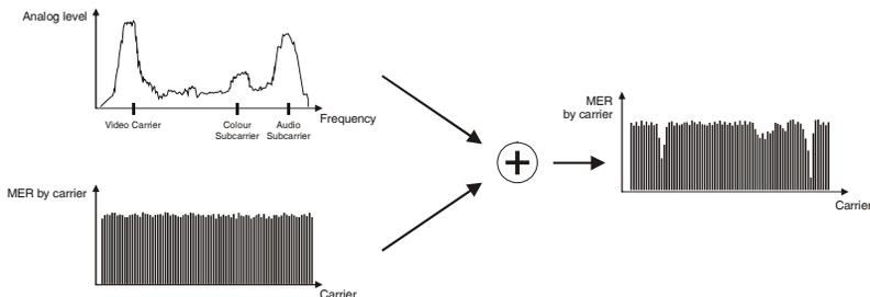
Figure 49.- Scheme of interference due to TV analogue signal over a digital channel.
