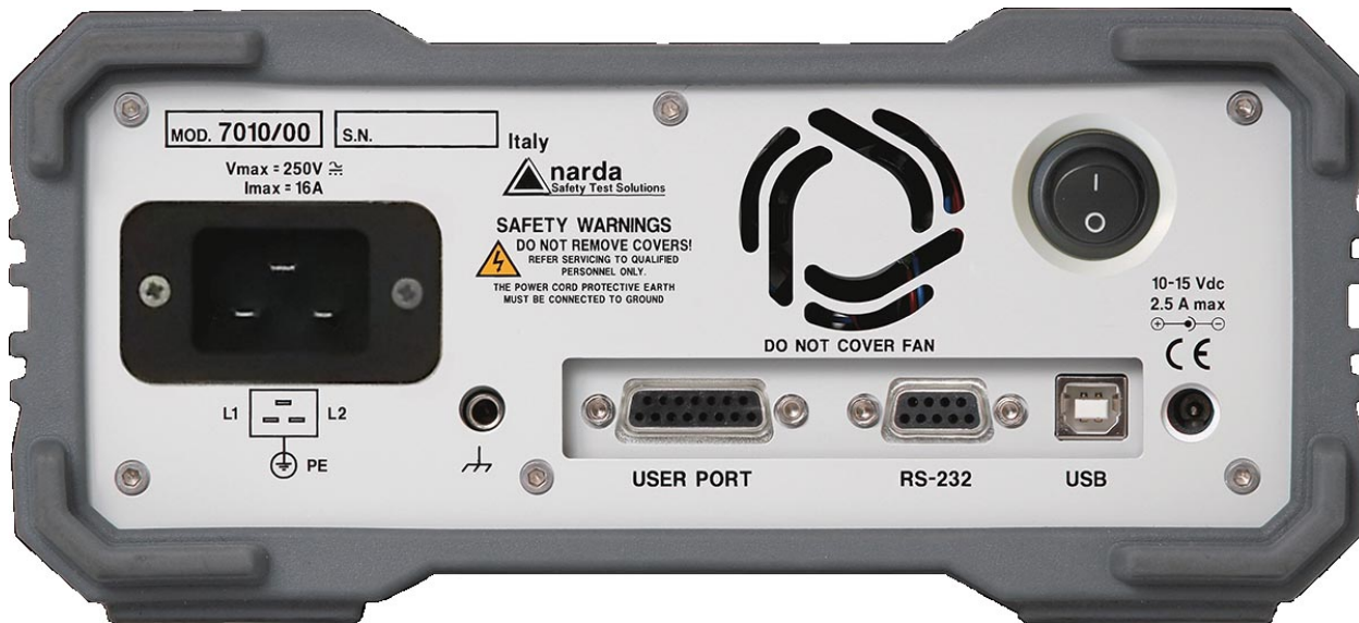
Fig. 1-2 7010 Option 00 Rear Panel
