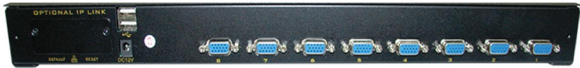
5. Using the included power adapter, connect the 12 VDC jack on the rear panel of the switch module (above) to an A/C outlet. **NOTE:** When the control platform is pulled out to its full extension, the bracket guides lock automatically and the power is turned on to the console.
