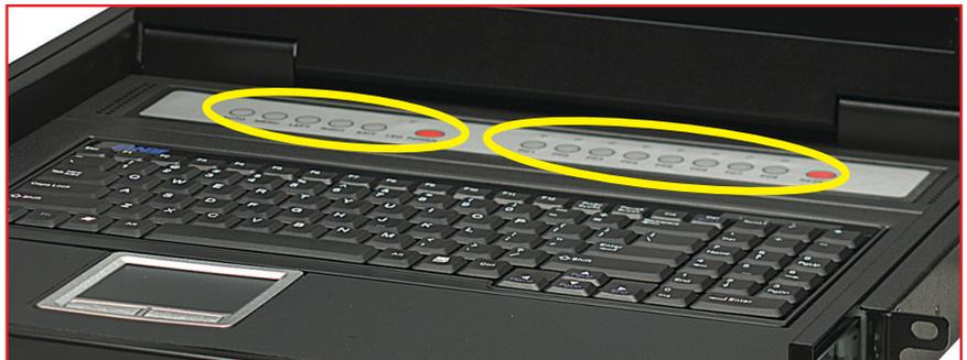
Also located on the control platform is the touch pad (below the space bar), which can be used instead of a mouse for on-screen navigation.
