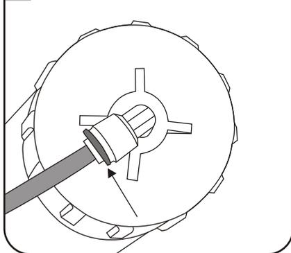
4 Remove the membrane housing cap anticlockwise.
