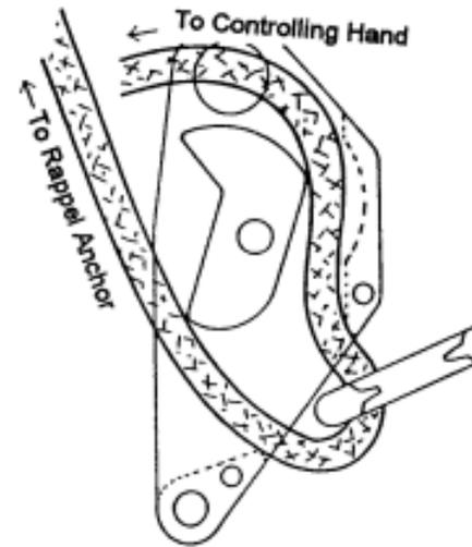
The rope can run either way when rappelling
