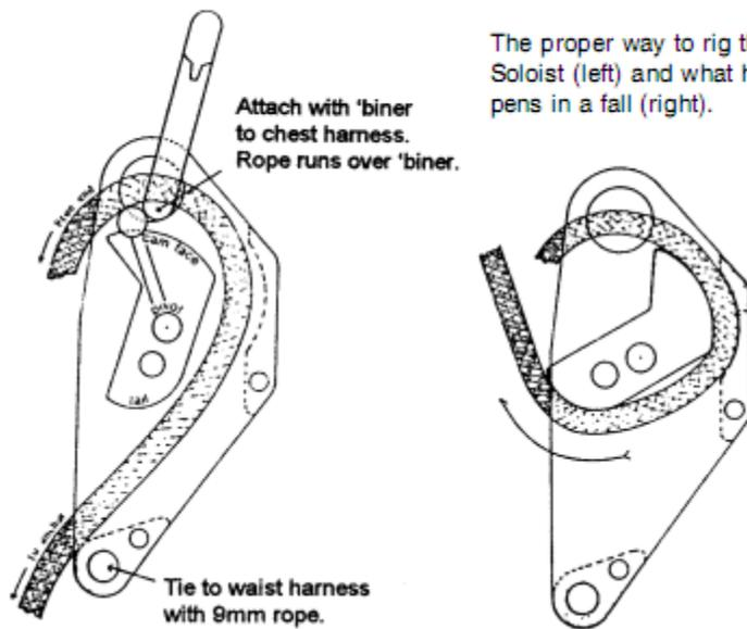
The Soloist relies on the direction of rope pull to lock it. The critical angle is the angle that the rope comes out of the Soloist. It will not lock if you fall headfirst.
