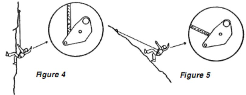
The falling climber's body position is identical in both of these cases. But the angle of the rope coming out of the Soloist is **not** the same.
