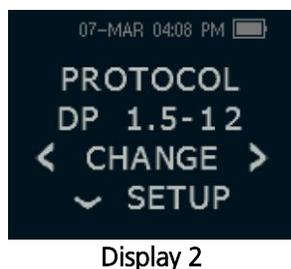
The currently selected protocol is shown on the Main Menu (Display 1). To change the selected protocol press ▼CHANGE at the Main Menu. The Change Protocol display will appear (Display 2). Use the ◀CHANGE▶ arrow buttons to change the selected protocol. Press the ▲UP arrow to return to the Main Menu to begin testing. Press the ▼SETUP to enter the setup menus.
