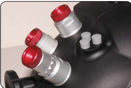
One way valve installed in 3rd bulkhead
