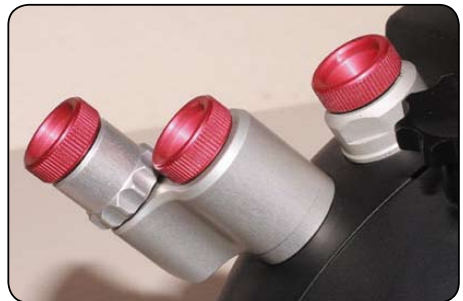
One way valve installed in manifold
