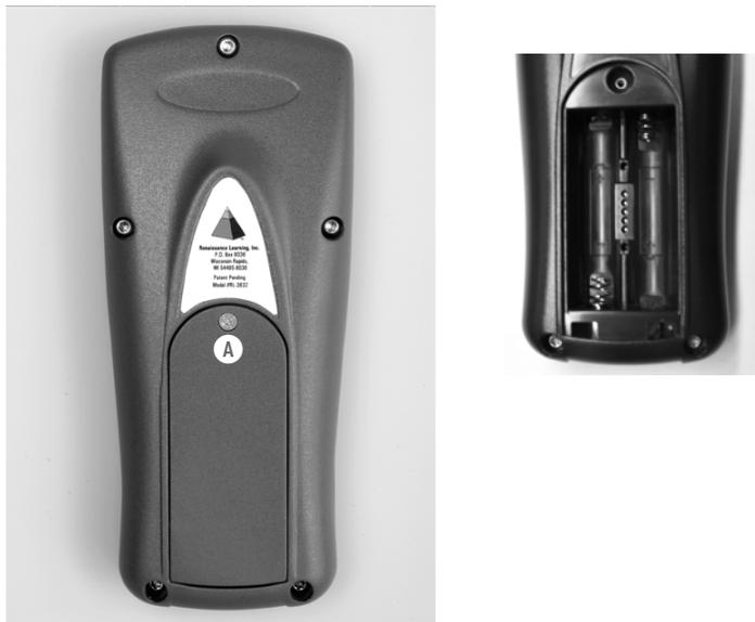
2. Remove the old batteries. Install two new ones, making sure the + and – ends are oriented as marked in the compartment.
