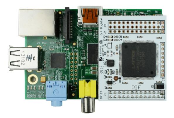
This is the documentation for Bugblat's Raspberry Pi FPGA board - the pif board.
