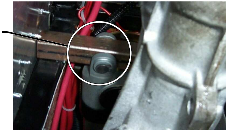
Figure 2.10. The clutch actuator viewed from underneath the car. Behind the aluminium gearbox, the mounting of the actuator is seen.
