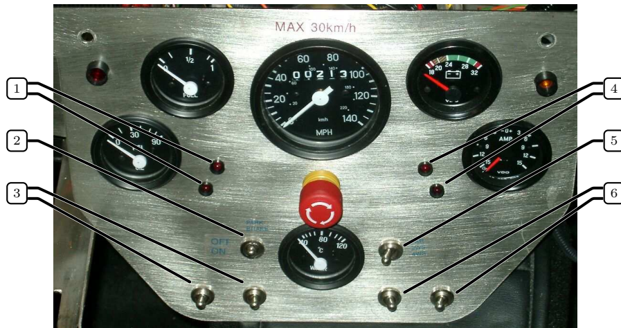
Figure 2.4. The dash board with switches. The upper left one is the parking brake switch (no. 2) and is connected to Node CL. The rest of the two-way switches (no. 3, 6), as well as the single three-way switch (no. 5), are connected to Node CR, and their function is controlled by the software implementation in the PowerNode. The same is true for the four LED:s (no. 1, 4), located just below the gauge indicators.
