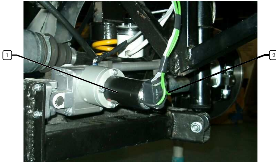
Figure 2.7. The rear right steer actuator DC motor (no. 1). The encoder (no. 2) is seen mounted on the outer end of the motor axle.
