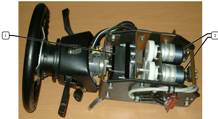
Figure 2.14. The movable steer module. The steering wheel MR-brake (no. 1) is seen in the middle of the module, and the two absolute encoders (no. 2) are found further to the right in the figure.
