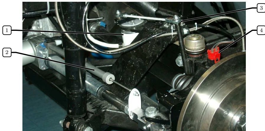
Figure 2.17. The figure shows the rear right encoder (no. 1) with linkage (no. 3) to the spindle, the linear position sensor (no. 2) on top of the ball screw actuator, and the speed sensor (no. 4) fitted inside the spindle (partly concealed by the brake disc).
