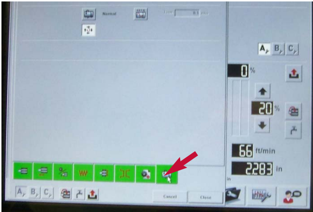
16. Press Spindle Options Icon, next icon on bottom bar. Accept Spindle Options setting. No action required. Spindle Option Icon, on bottom bar will be green.
