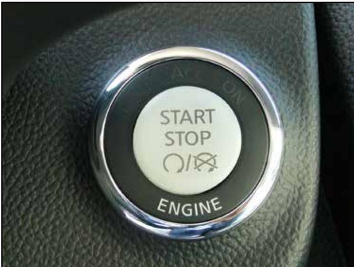
**1)** The car has a “PUSH” Button to start the engine instead of a mechanical ignition.
