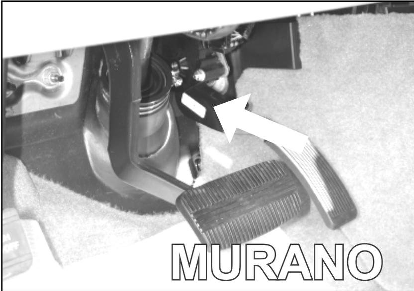
The Murano uses a Random PIN Code that must be converted from the serial number on the BCM (Body Control Module) which is located under the dash to the right of the steering column.
