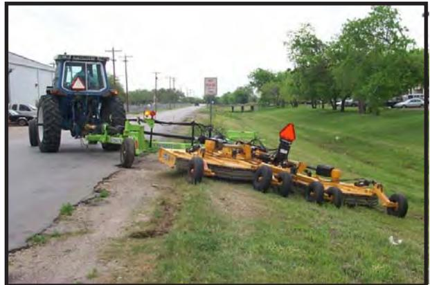
To avoid overturns, drive the tractor with care and at safe speeds, especially when operating over rough ground, crossing ditches or slopes, and turning corners. Rear tractor tire spacing should be increased when working on inclines or rough ground to reduce the possibility of tipping. Utilizing the flex arm will increase safety during operation. The tractor does not have to ride on the ditch slopes there by reducing the possibilities of a rollover.
