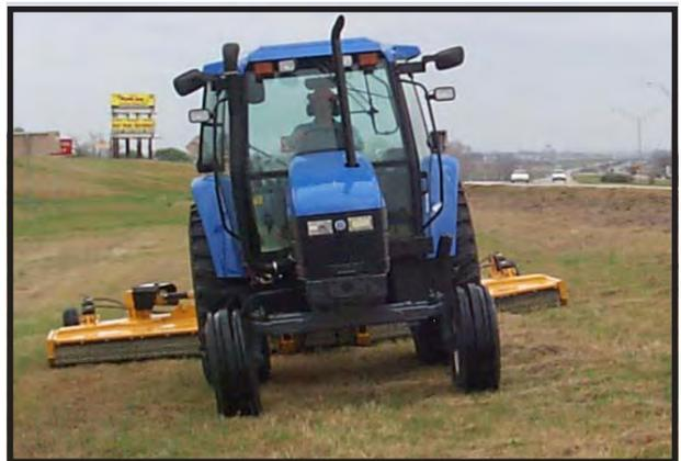
Use extreme caution when operating on steep slopes. Keep the tractor in a low gear when going downhill. DO NOT coast or free-wheel downhill.
