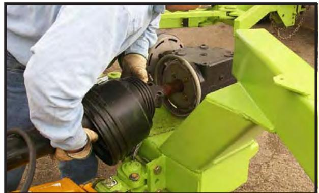
**IMPORTANT:** DO NOT use a non-CV tractor shaft. Driveline damage will occur when turning the implement.
