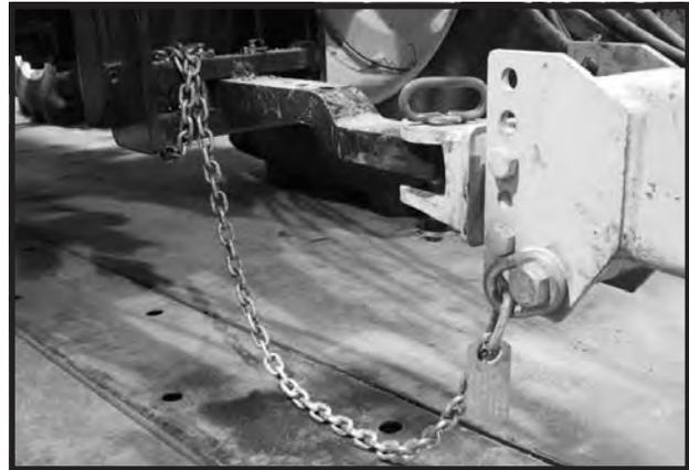
**WARNING!** Do not use safety tow chain for towing. Replace entire chain if any link or end fitting is broken, stretched, or otherwise deformed.
