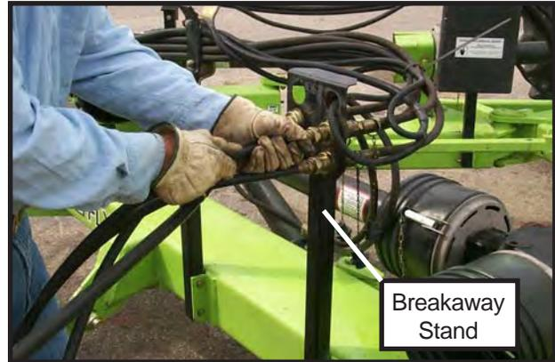
The selector valve kit reduces the required tractor ports and provides double acting wing lift action.
