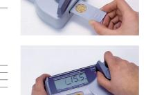
First, confirm that the figures "8 TIMES 88.8%" and several other marks appear when the "POWER" button is pressed with your finger. Should the figures not appear ,or any mark,the batteries are exhausted. Replace all of the batteries with new ones, according to the diagram illustrated in the battery chamber.
