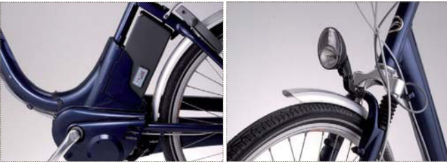
Giant bike uses the Panasonic drive with Ni-Mhd battery, time-tested for years. Rather comfortable: Thanks to twilight sensor the hub dynamo light goes on automatically, when needed.
