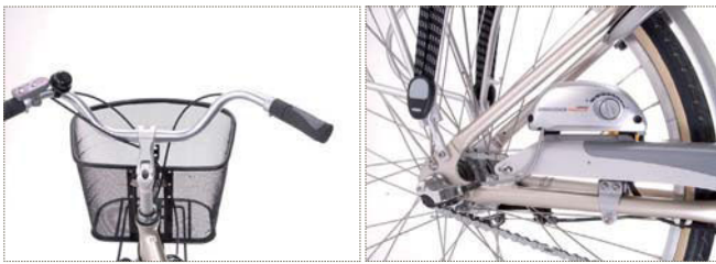
Neat cockpit and a big basket at the handlebar At loose pedalling the Shimano-Auto-D gear shift provides the right gear. Only when changing into lower speeds it takes too long to shift.
