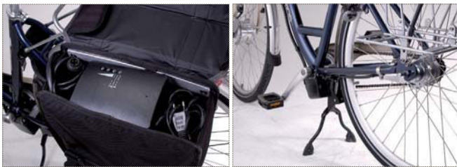
Convenient: the charger can be placed in the saddle bag above the battery. Solid: Sram hub gear shift and Sanyomotor and torque sensor
