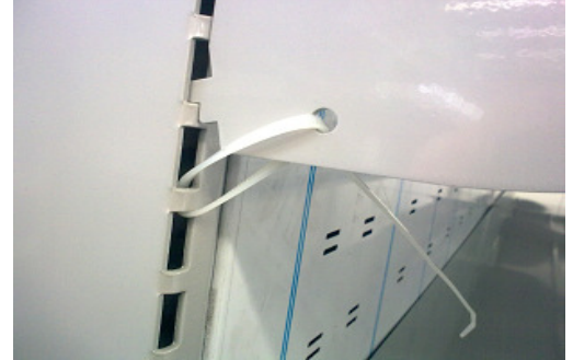
Remove plastic shelf clips (ties) with a knife or scissors if any
