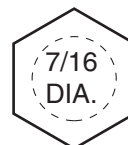
7/16" Bolt or Nut Wrench (Bolt)—5/8" Wrench (Nut)—11/16"
