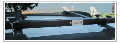
Center your single scull rack from front to back on your vehicle roof racks. Use the included U-bolts to attach the single scull rack to your vehicle racks. Make sure the u-bolts face opposite directions.
