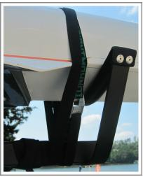
If you have excess webbing from the straps, make one more wrap around the hull of the boat and then wrap the remaining webbing around the main rail of the single scull rack. Tie off the last few inches so that the webbing does not flap in the wind during travel. If you prefer to make the webbing extremely secure, you can use a couple wraps of electrical tape to secure the loose end of the strap.
