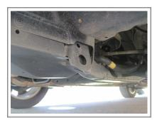
We recommend lining up your single scull rack with the towing hooks located underneath your car's undercarriage. These hooks are often located to the left and right sides of your vehicle. They will provide tie down points later for your bow and stern lines.
