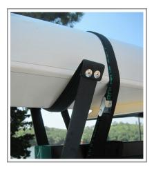
Use (2) boat straps to secure your boat to your single scull rack. Straps should be located directly to the inside of the front and rear cradles so that they wrap around the boat and the main rail on the single scull rack. Straps should be pulled tight enough so that they are snug and so that the boat pulls down into the cradles.
