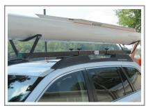
Do not transport your boat cockpit up. Our single scull roof racks were designed to transport boats by the decks of the boat, which are much flatter than the hull of the boat. Transporting your boat cockpit up will result in unnecessary rocking and movement from side to side during travel. Transporting cockpit up will also potentially allow for the collection of rainwater.
