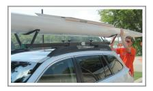
Slide the hull of your boat forward onto the rack until the cockpit of your boat is centered between the front and rear cradles. For taller vehicles, you may have to position a step ladder near the bumper of your vehicle to assist with loading.
