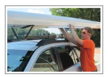
This is the most common method to load/unload. Find the center balance point of your de-rigged scull and then carry it overhead to your vehicle. Place the decks of the scull in the cradles of your roof rack one at a time, making sure that the cockpit of your boat is centered between the cradles of the roof rack.
