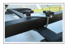
Tighten the lobed knobs on the U-bolts so that the plates bend over the rail of the single scull rack. Once tightened, grab the rail of your single scull rack and shake. It should move the entire car such that you hear your gas tank sloshing.
