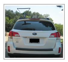
If you are only transporting one boat, we recommend locating your single scull rack to one side of your car. Your vehicle racks are stronger towards the ends, so positioning your load over the ends will result in a more stable attachment point. This will also make it easier to load/unload your boat.
