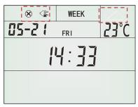
Registering, No GSM signal, AC/DC adaptor lost.
