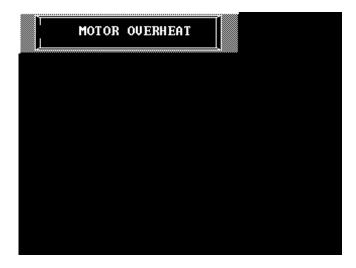
The motor overheat is displayed in the motor status window when the motor is overheated. To reset the whole machine must be turned off. This allows the controller to download reset commands to the motor's control circuits
