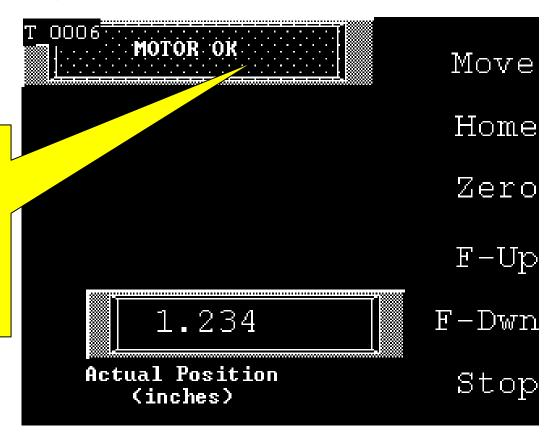
Motor Diagnostic: Continually monitors motors conditions. This is were Upper limit and lower limit alarm will be displayed. As well as a motor overheat condition alarm.
