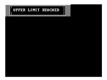
The "UPPER LIMIT" or "LOWER LIMIT" will be displayed in the motor status window when the platen reaches it's mechanical travel limit. There are mechanical limit switches inside the steel cross bar and these are wired directly to the servo motor.
