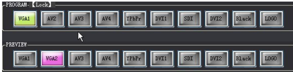
Fig 4.6 Signal switching area
