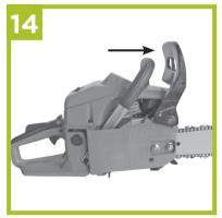
**Note:** The brake lever should snap into both positions. If strong resistance is felt, or lever does not move into either position, do not use your saw. Take it immediately to a professional Service Center for repair.
