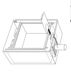
10. Turn the clamping plate up-side down and slide the plate between the guides so that its ends grip around the pipe opening (see fig. 10). Make sure that the flue collar plate is pressed onto the burner chamber.
