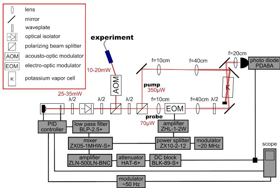
**Figure 7:** Laser Lock Setup. For reasons of simplicity most mirrors that are necessary for beam alignment are not shown in this schematic. Electronics from minicircuits are shown with part numbers.
