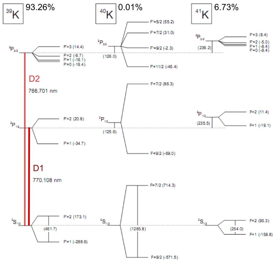
**Figure 3:** Energy level structure showing the D1- and D2-line of the potassium isotopes  $^{39}\text{K}$ ,  $^{40}\text{K}$  and  $^{41}\text{K}$  from [4].
