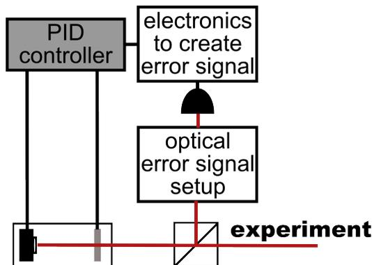
**Figure 4:** Principle of a laser lock setup. A small part of the laser intensity is used to create an optical frequency dependent signal that is detected and manipulated electronically to create a linear frequency depend error signal that is fed back to the laser to correct for the frequency aberration.
