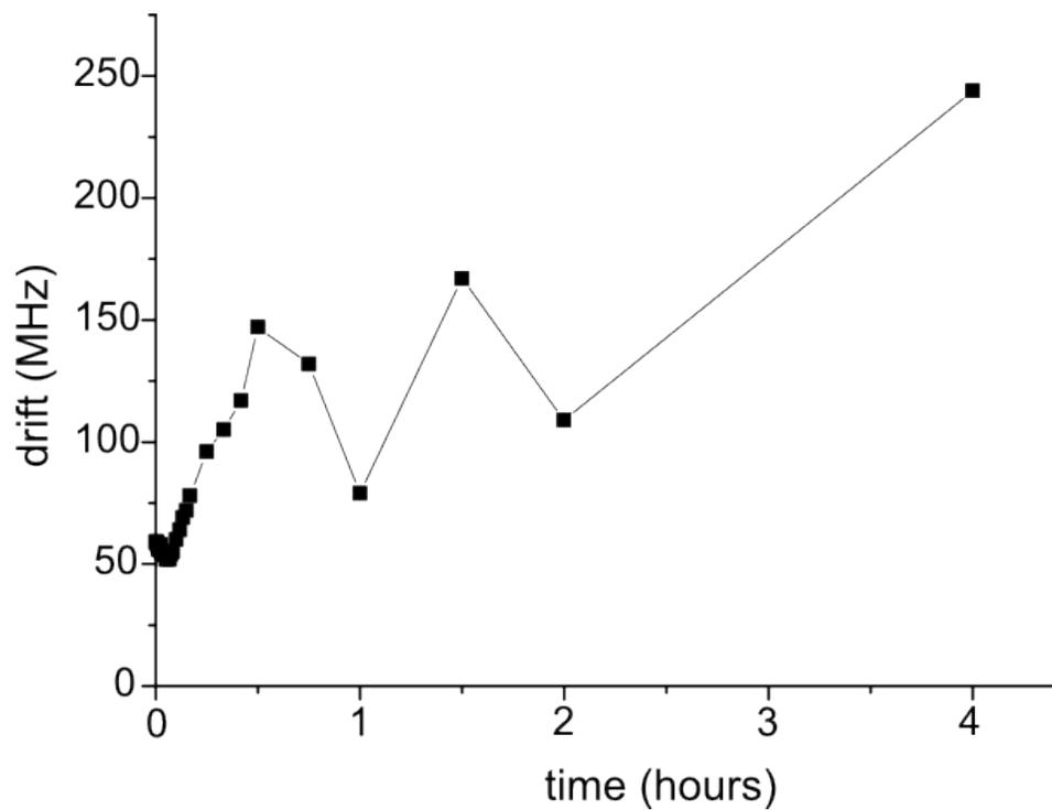
**Figure 10:** An exemplary measurement of the frequency drift of the unlocked laser 3 with the spectrum analyzer in a beat measurement against a locked laser from another experiment.
