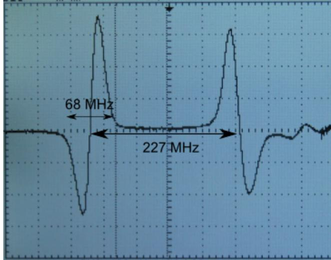
**Figure 9:** Frequency depend error signal with frequency scale. The frequencies refer to the distance between the tips of the arrows. The two peaks correspond to the  $F = 2$  transition (left) and the crossover (right) between  $F = 1$  and  $F = 2$
