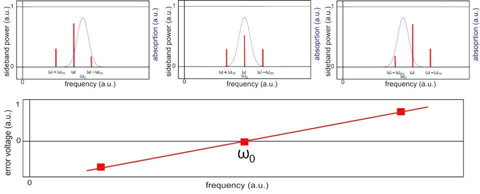
**Figure 6:** The three upper graphs show the sideband attenuation for different frequencies of the main peak with the corresponding DC-error-signal underneath.
