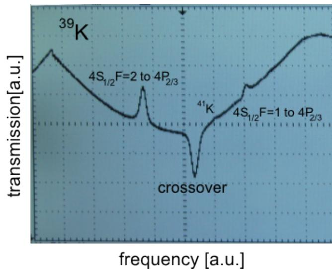
**Figure 2:** Saturation absorption spectroscopy signal of our setup.  $F = 1$ ,  $F = 2$  and crossover peaks of the  $^{39}\text{K}$  D2-line are labeled (see potassium energy levels D1 and D2-line in figure 3).  $^{41}\text{K}$  isotope peaks are barely visible. We don't subtract the single beam doppler peak because it doesn't contribute significantly to the error signal (see section 2.2.) (which is proportional to the first derivative of the saturation signal).
