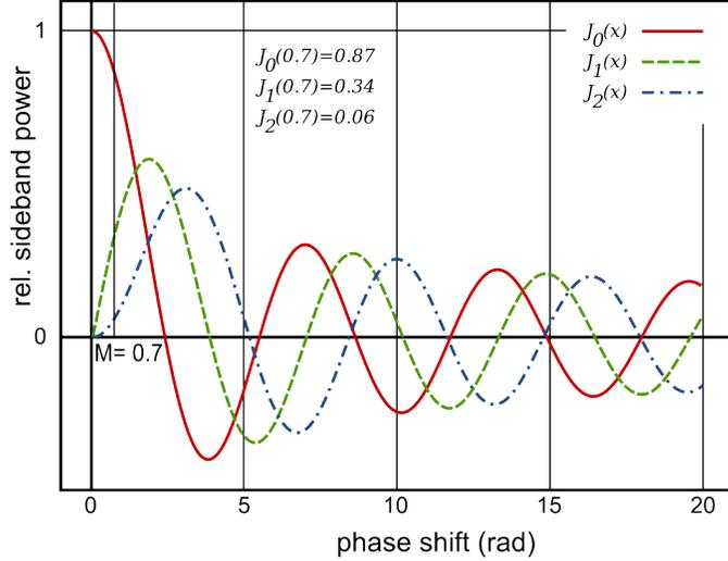
**Figure 5:** First three order Bessel functions. Vertical line shows modulation depth in our setup at  $M \approx 0.7(\text{rad})$ .
