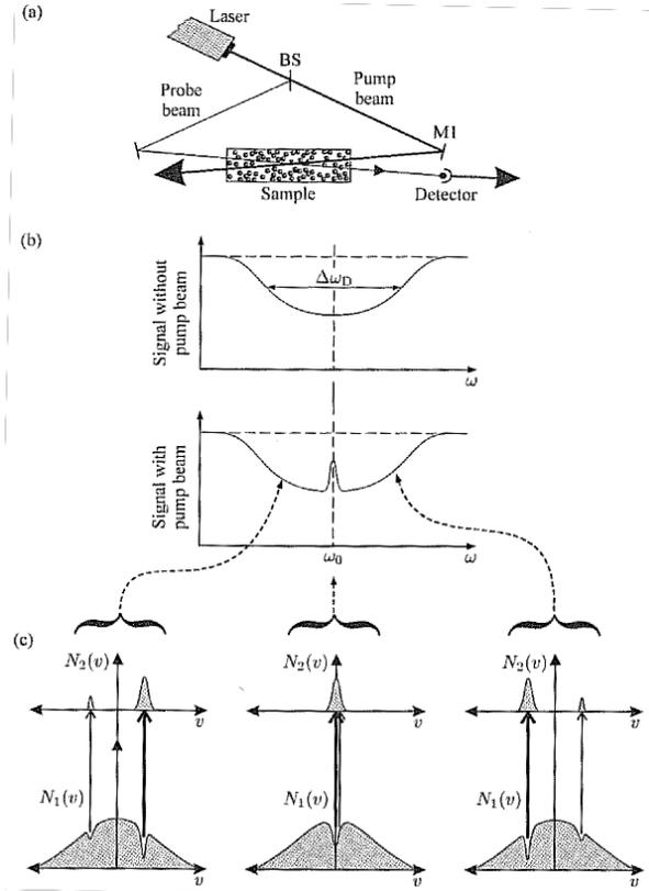
**Figure 1:** A saturated absorption spectroscopy (SAS) experiment [5]. a) Basic SAS setup. b) Shape of photo diode signal without and with pump beam. c) Velocity (only component in beam direction) distribution of atoms in a two level system with increasing beam frequencies from left to right hitting the resonance in the center. Positive velocities are defined in probe beam direction. The thick arrows are pointing out the higher intensity of the pump beam.
