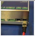
The Ethernet interface is the rightmost connector.
