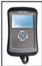
Cortex with programming cable plugs into your vehicle's OBDII port under your steering wheel & dash.
