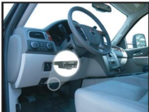
Cortex programming cable plugs into your vehicle's OBDII port under your steering wheel & dash.
