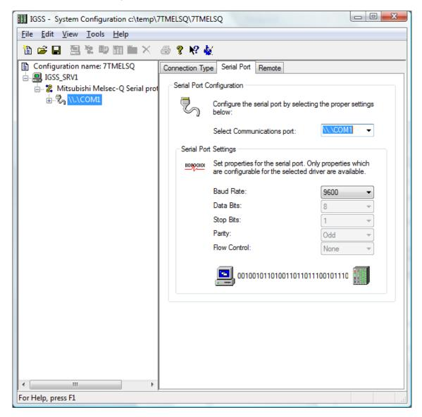
Since the Mitsubishi Melsec Q protocol is designed for point-to-point communication you need one serial port for each PLC you connect to. The IGSS Mitsubishi Melsec Q driver supports up to 8 serial ports (8 PLC connections).
