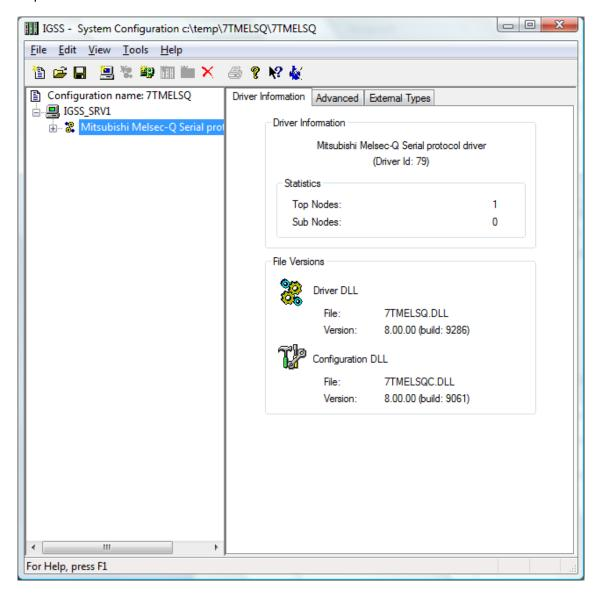
Once the driver has been added to the relevant station then you are ready to proceed with adding PLC nodes. This is done by right-clicking on the driver and select "New Interface" menu point.
