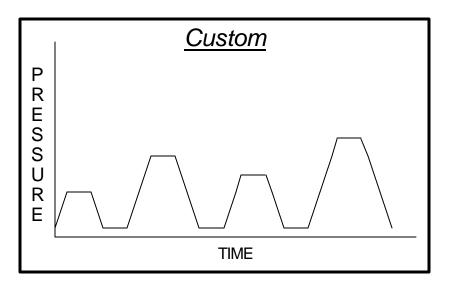
This is a custom pressurization profile. It works like Incremental mode, except that each successive *Target Pressure* is defined individually. Up to 100 successive Target Pressures can be defined for a given test. These custom target pressures need bear no relationship to each other; one target may be greater than, less than, or equal to any of its neighboring targets.
