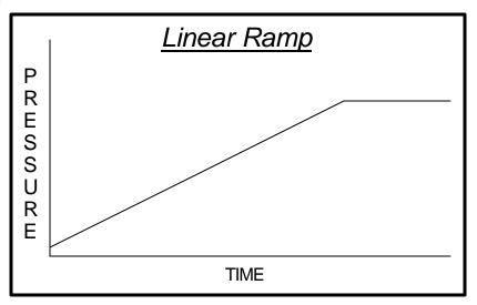
Continuously increasing pressure is applied to a product until it reaches its *Target Pressure*, then stays at that pressure for the *Dwell Time*, or until a burst or leak is detected.
