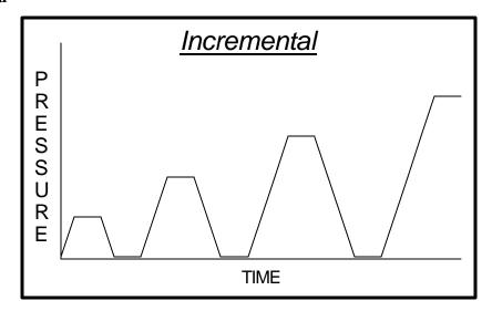
Pressure increases to programmed *Target Pressure* and stays there for the specified *Dwell Time*. If no burst or leak occurs, the pressure is decreased to the specified *Return Pressure* level. This repeats a specified *Repeat Cycle* number of times. Once the *Repeat Cycles* complete, a new *Target Pressure* is computed by increasing the previous pressure by the *Pressure Increment* amount. The test continues like this until a burst or leak, or the *Maximum Pressure* is achieved.
