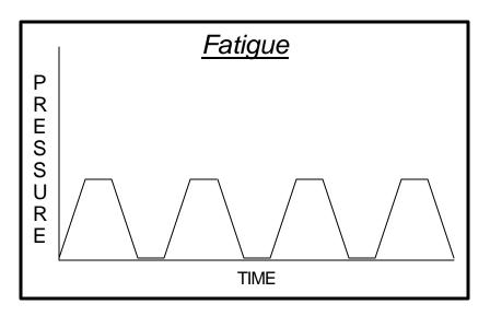
The Fatigue mode repeats a single defined pressurization *cycle*. Pressure increases to a programmed *Target Pressure*. Product will remain at pressure for the specified *Dwell Time*, and then de-pressurized to the *Return Pressure*. This repeats for the *Repeat Cycles* defined for the test.
