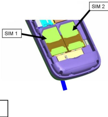
Keep the metallic face of a SIM card downward, and slide it gently to the position of SIM 1.
