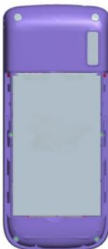
**Install:** Match the metal contacts of battery separately with the battery compartment metal contacts, and put the battery base into the slot;
