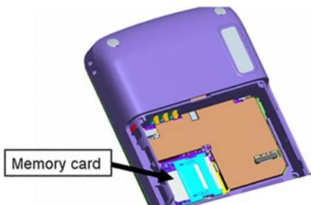
Keep the metallic face of a memory card downward, and slide it gently to the position of Memory card.
