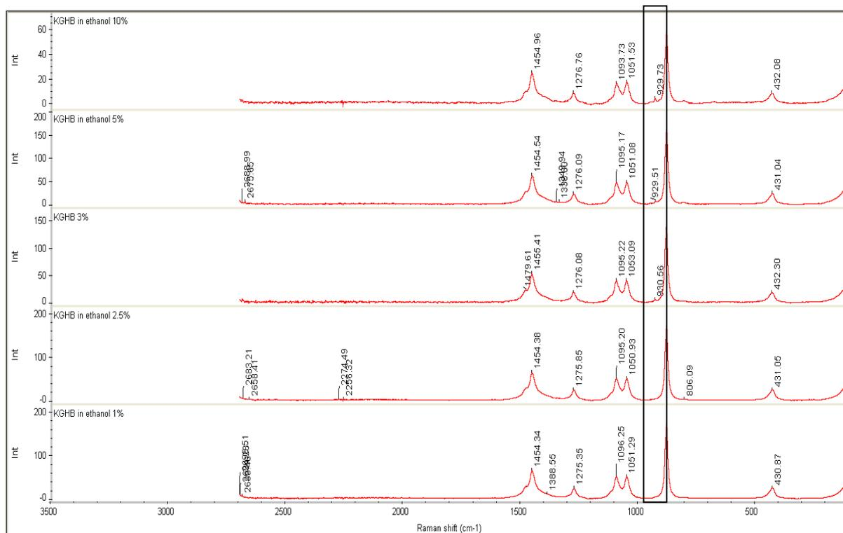
Figure 1.10: KGHB limit of detection in ethanol.
