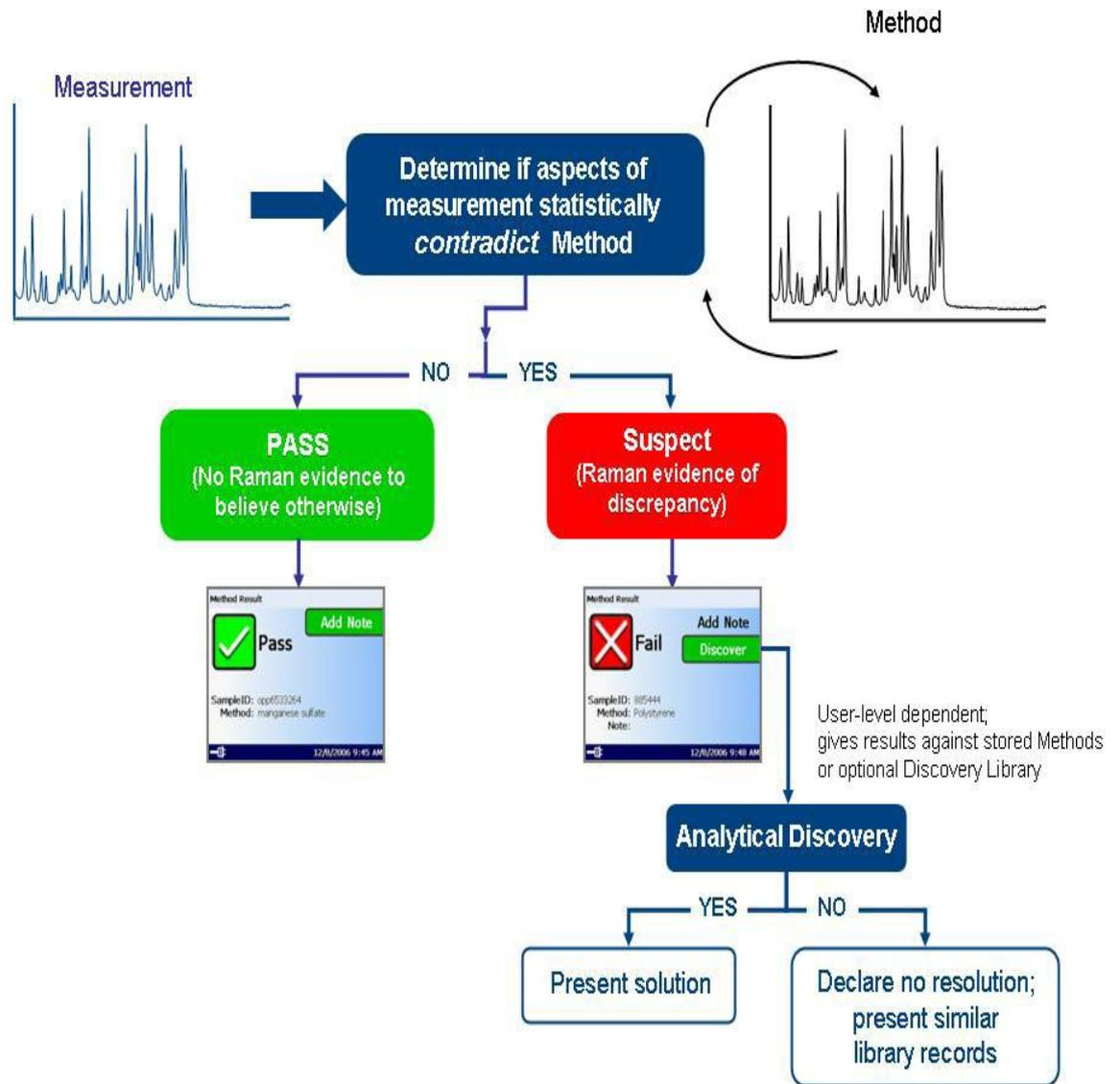
Figure 1.11: TruScan PASS/FAIL System (TruScan user manual, 2010)
