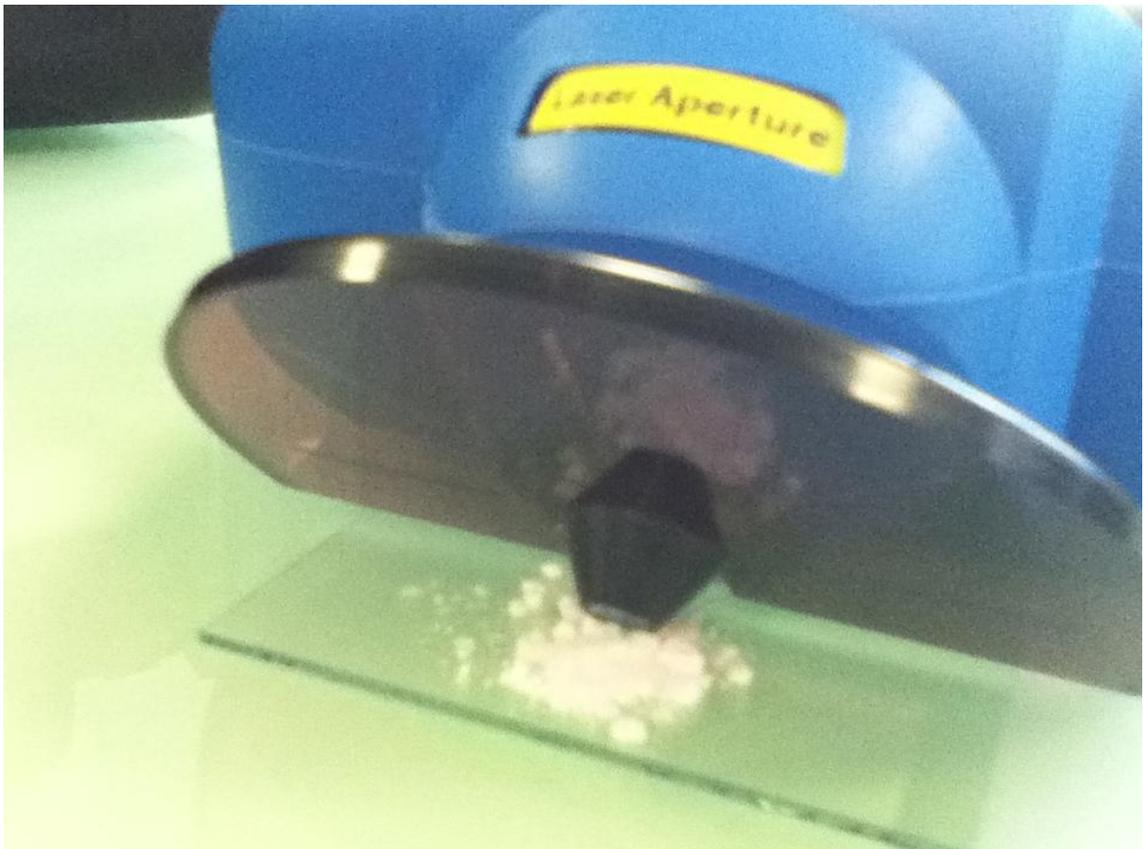
Figure 2.3:TruScan focussed on white powder. This figure demonstrates how the powder was presented to the TruScan device. It was put onto a glass slide, with all the powder in one concentrated area of the slide and the nose cone was very close to the powder when a run was carried out.
