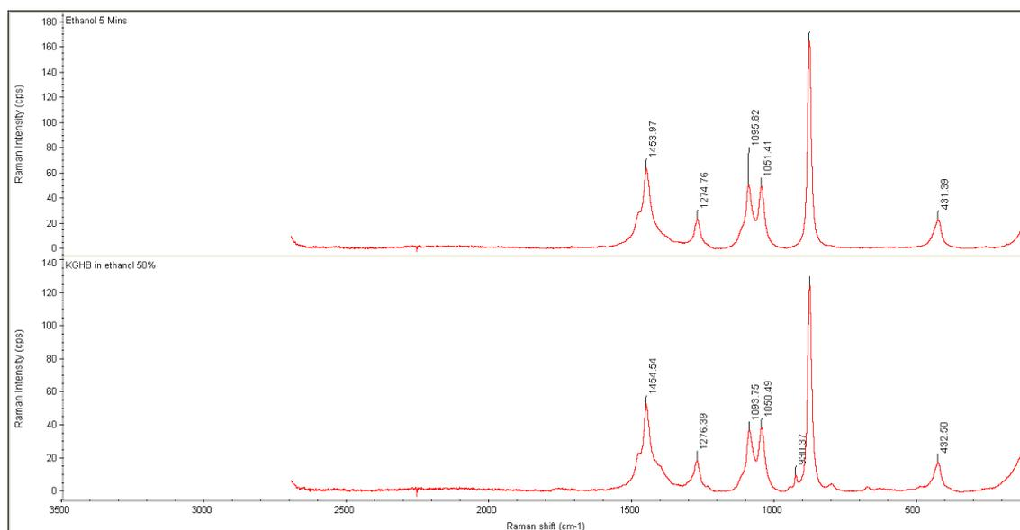
Figure 1.9: KGHB in Ethanol compared to neat ethanol spectra
