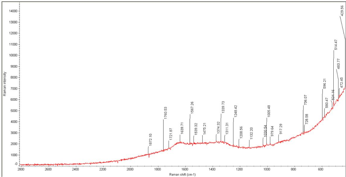
Figure 3.14: 2 mg amphetamine sulphate in 1 mL oral fluid
