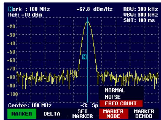
The R&S FSH3 now displays the counted marker frequency with a resolution of 1 Hz. To indicate that the **FREQ COUNT** function is on, **Mark** in the top left corner of the screen changes to **Count:**
