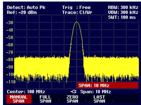
Use the FULL SPAN softkey to select the full Span from 0 Hz to 3 GHz with a single keystroke.
