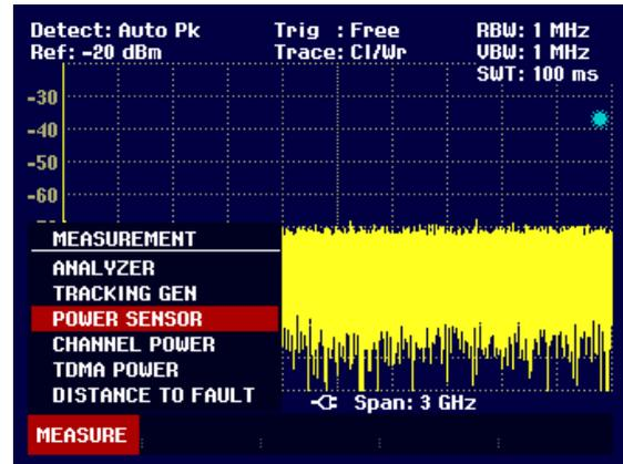
The R&S FSH3 opens the screen for power measurements. If a power sensor has not been connected, no measured value is displayed. If a power sensor has been connected, the R&S FSH3 sets up a connection via its interface and after a few seconds displays the measured power.
