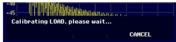
When calibration is over, the R&S FSH3 displays **DTF CAL** in the top right-hand corner of the screen. The REFLECT CAL softkey label is highlighted in green to indicate that calibration has been successfully completed.
