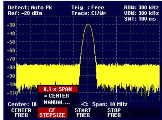
If you select "0.1 x SPAN" or "= CENTER", the R&S FSH3 makes the setting directly itself. If you select "MANUAL...", the value entry box opens and indicates the current stepsize.
