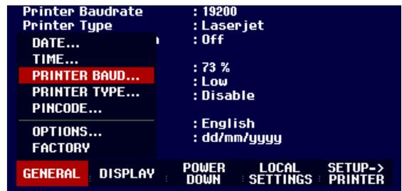
The selection box for the baud rates available (1200 baud to 115200 baud) opens.
