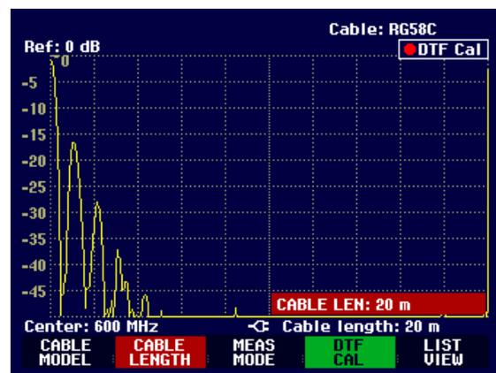
*N.B.: The cable length should be entered before the test setup is calibrated. If it is entered afterwards, the measurement accuracy is reduced.*
