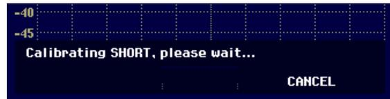
When calibration is over, the R&S FSH3 outputs the message "Reflect. calibrated" for 3 seconds.
