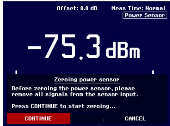
When zeroing is over, the R&S FSH3 outputs the message "Power Sensor Zero OK" and switches back to the softkey menu for the power sensor.
