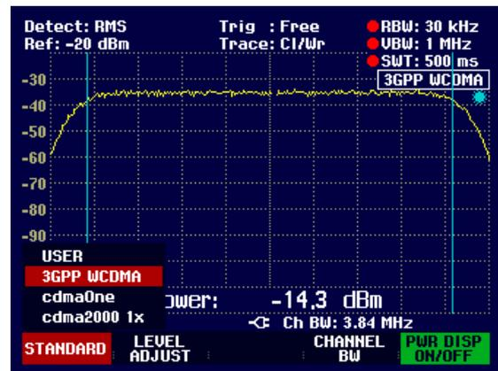
If USER is selected, the R&S FSH3 sets the last channel power measurement setting used in the USER mode. The R&S FSH3 automatically makes changes to the setting so that it is again available when the USER standard is called again.
