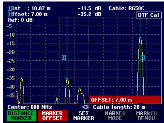
As is the case with spectrum analysis, the R&S FSH3 provides functions to automatically position the marker or the marker offset on the trace. These can all be accessed by pressing the SET MARKER softkey.
