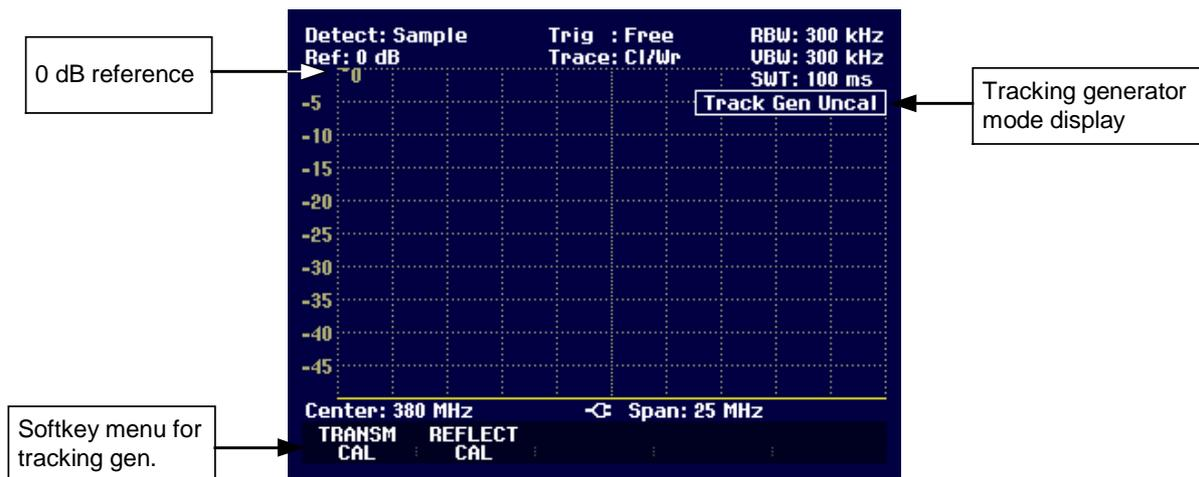
When the tracking generator is switched on, the R&S FSH3 displays **Track Gen Uncal**. This indicates that tracking generator measurements are uncalibrated. The level axis is in the relative unit dB. Apart from the level values, the 0 dB reference is also displayed. This corresponds to a reference level of  $-20$  dBm in the Spectrum Analyzer mode (= nominal output level of the tracking generator).
