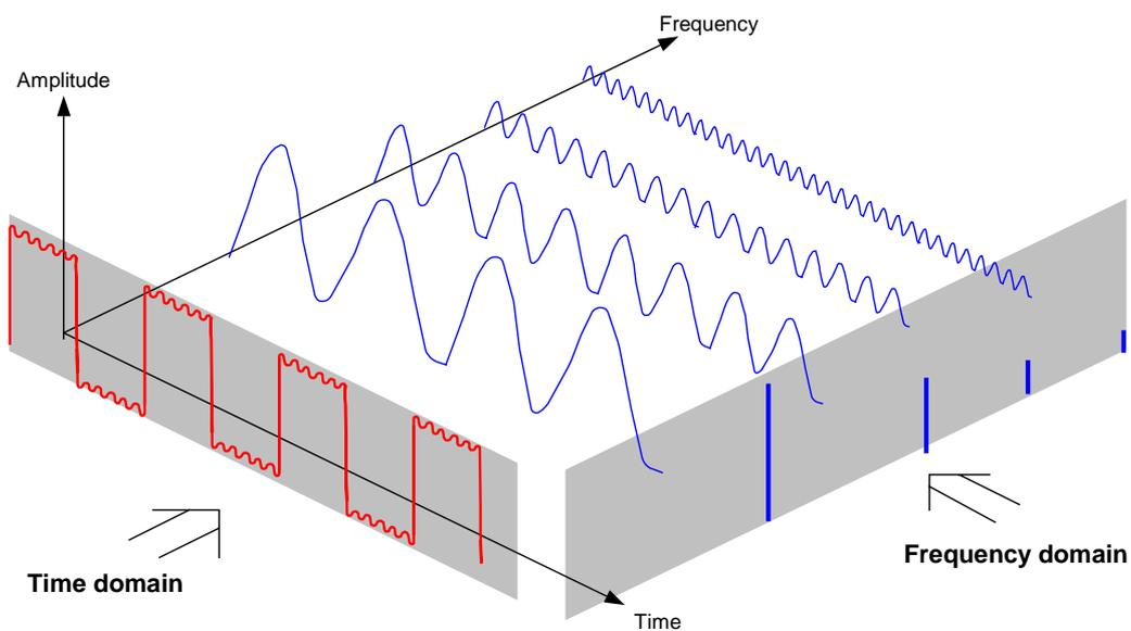
The periodic squarewave in the time domain can be Fourier transformed to the frequency domain. In the case of a squarewave there is a fundamental (= frequency of the squarewave) and its odd harmonics. Using a narrow bandpass filter, the Spectrum Analyzer makes measurements in the frequency domain. Only at frequencies where there is a signal is there a reading which gives the amplitude of the frequency component.
