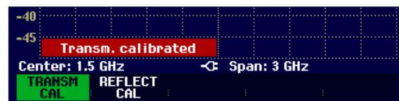
The R&S FSH3 displays now **Transmission** in the top right-hand corner of the measurement diagram. This tells the user that the R&S FSH3 has been calibrated for transfer function measurements.
