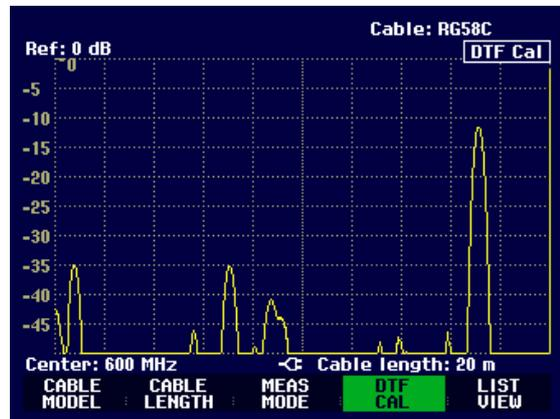
The R&S FSH3 can also list any cable faults. It displays the return loss and distance from the measurement plane of all reflections that exceed a settable threshold.
