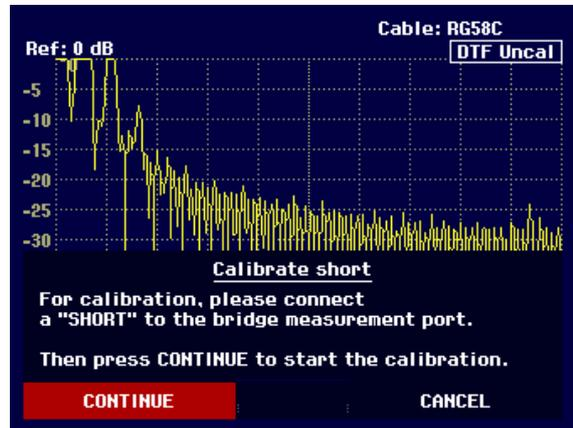
While SHORT calibration is in progress, the R&S FSH3 outputs the message "Calibrating SHORT, please wait...".
