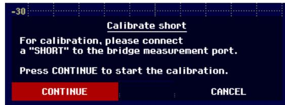
When calibration is over, the R&S FSH3 outputs the message "Reflect. calibrated" for 3 seconds.
