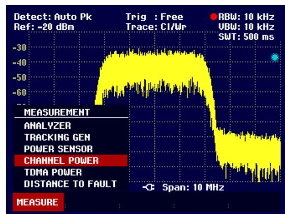
The R&S FSH3 displays the softkey menu for setting the channel power measurement. Two vertical lines in the measurement diagram indicate the channel bandwidth. The measured channel power is shown in large letters below the measurement diagram.
