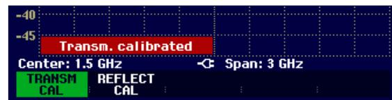
When calibration is over, the R&S FSH3 displays **Transmission** in the top right-hand corner of the measurement diagram. This tells the user that the R&S FSH3 has been calibrated for transfer function measurements. The softkey label **TRANSM CAL** is highlighted.
