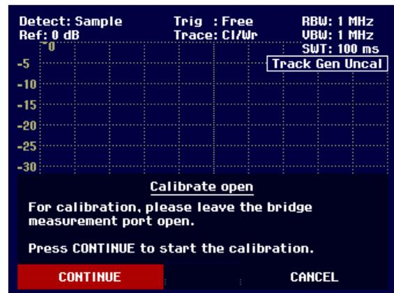
When OPEN calibration is over, the R&S FSH3 prompts the user to perform SHORT calibration.
