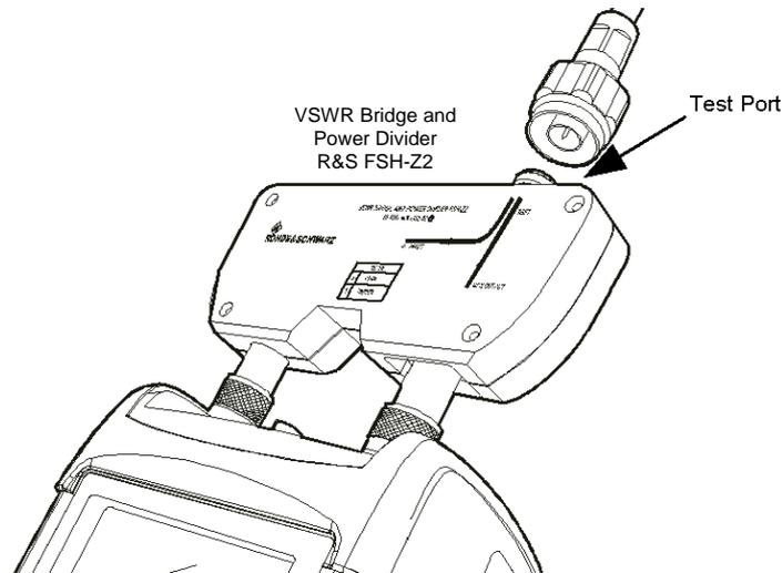
The R&S FSH3 can measure both a DUT's return loss and its VSWR.
