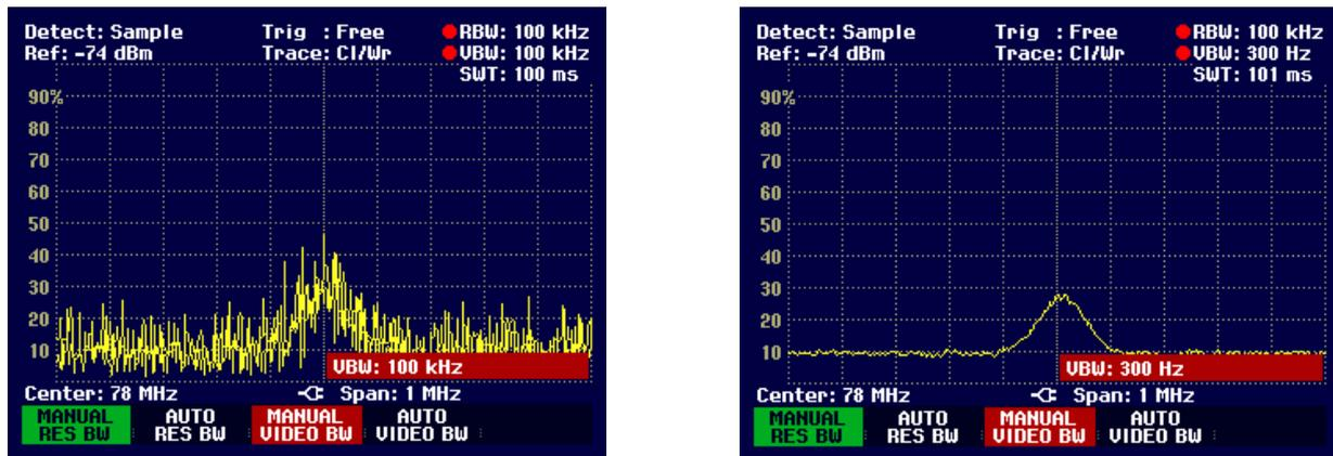
Limiting the Video BandWidth smoothes the trace considerably. This makes it much easier to determine the level of the measured signal.
