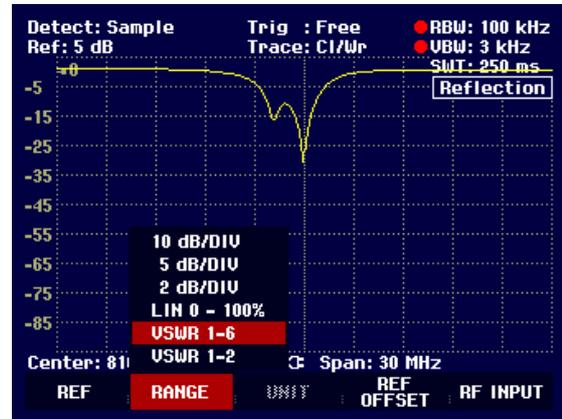
The R&S FSH3 displays the VSWR of the DUT.
