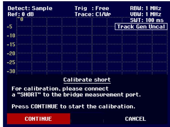
During calibration, the R&S FSH3 outputs the message "Calibrating SHORT, please wait...". Calibration can be aborted with the CANCEL softkey.
