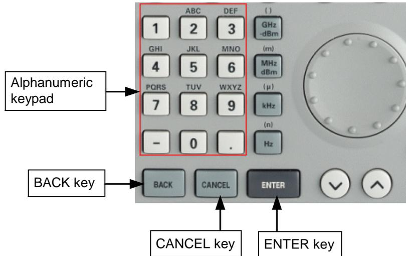
If the R&S FSH3 is expecting a letter entry, it automatically assigns the letters above the keys to the keys in the alphanumeric keypad. The keys have a multiple assignment. Enter the letter you want by pressing the key in question the appropriate number of times.
