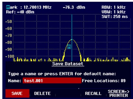
The dataset name comprises a text section and a numerical extension which are separated by a full stop. The dataset name suggested by the R&S FSH3 is derived from the last name to be used with the numerical extension incremented by 1.
