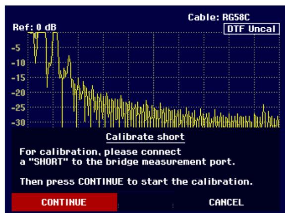
When SHORT calibration is over, the R&S FSH3 prompts the user to terminate the measurement plane with a 50 Ω Load.
