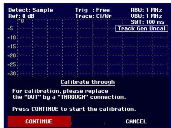
When calibration is over, the R&S FSH3 outputs the message "Transm. calibrated" for 3 seconds.
