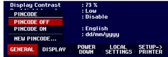
Use the Rotary knob or the Cursor keys to select the PINCODE... menu item and press the ENTER key. The selection box with the PIN code settings is opened.
