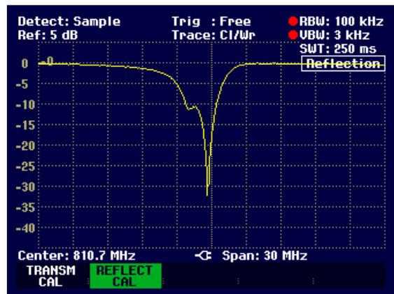
The transmission calibration remains valid until the R&S FSH3's Center Frequency or span are changed. If calibration becomes invalid, the R&S FSH3 displays Track Gen Uncal in the top right-hand corner of the screen.
