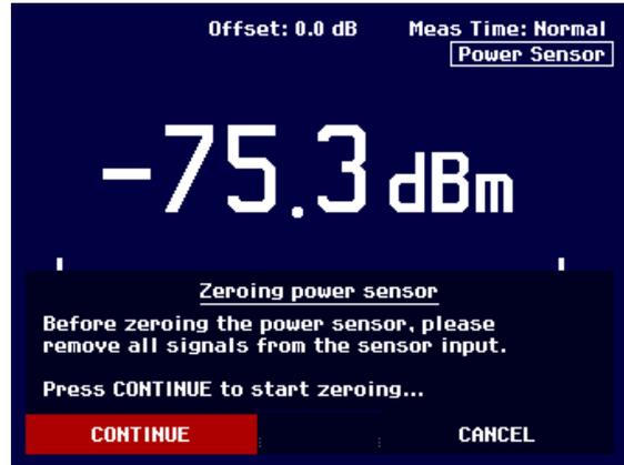
The R&S FSH3 immediately starts power meter zeroing. While this process is going on, the R&S FSH3 outputs the message "Zeroing power sensor, please wait..".
