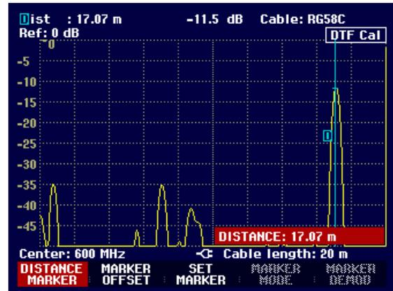
Checking the return loss of the cable under test:
