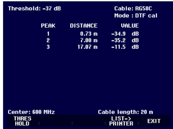
The distance to the cable faults or the distance between any two faults can also be read off with the marker.
