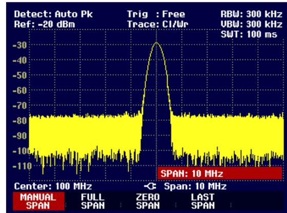
The R&S FSH3 has markers for reading off signal levels and frequencies. Markers are always positioned on the trace. Both the level and frequency at their current positions are displayed on the screen.
