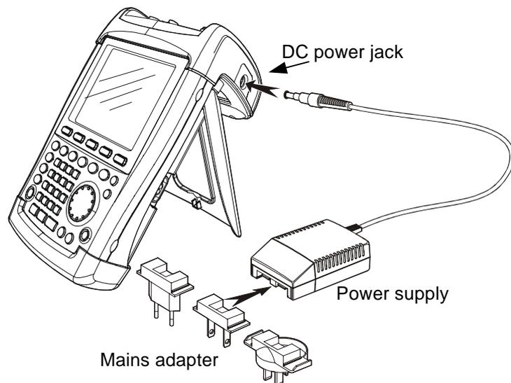
For rapid charging, switch off the R&S FSH3 during charging. The charging time is approx. four hours.
