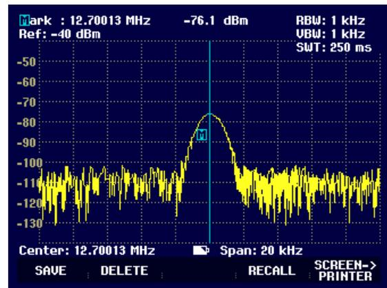
➤ The SCREEN->PRINTER softkey starts the screenshot printout on a printer.
