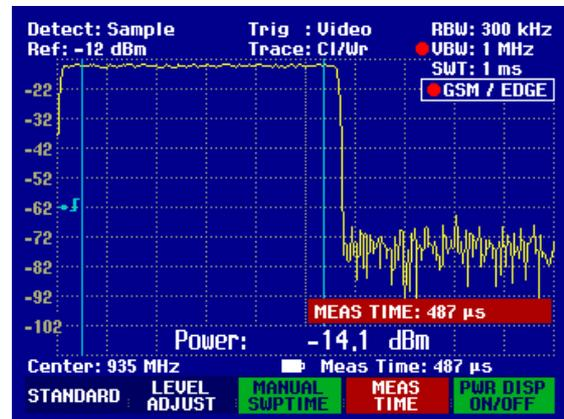
The minimum measurement time is the time corresponding to one trace pixel (= sweep time / 301).
