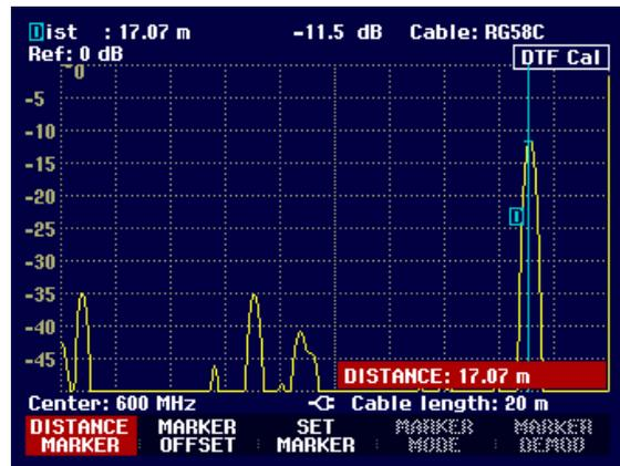
The reference plane to which the distance of a reflection is referred can be redefined using the marker offset.
