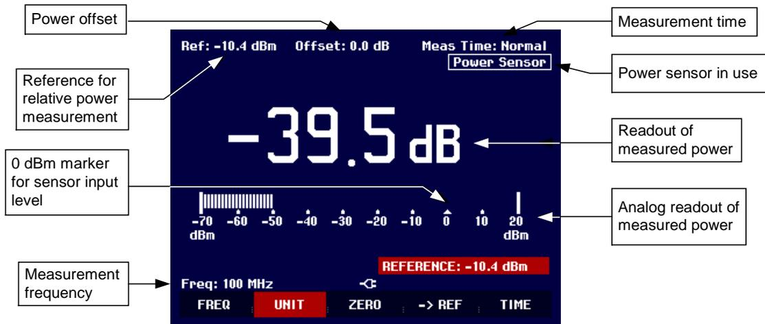
The power sensor has a memory containing frequency-dependent correction factors. This means that the highest accuracy is reached for signals whose frequency is known. If the R&S FSH3 switches over to the power measurement mode from another operating mode, it uses the Center Frequency as the frequency for the power sensor.
