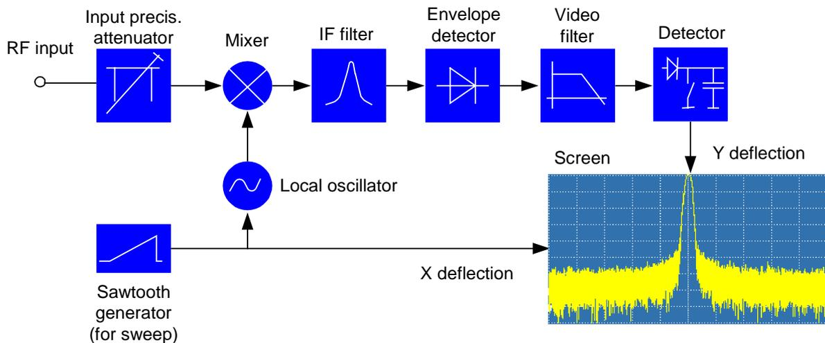
The precision attenuator at the input of the Spectrum Analyzer adjusts the level of the measurement signal to the level range that the mixer can handle without overdriving it. The precision attenuator at the input of the R&S FSH3 is adjustable in 10 dB steps from 0 dB to 30 dB and is directly coupled to the reference level setting.
