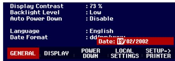
After the last data block has been entered, the R&S FSH3 verifies the validity of the entered date. If the date is not valid, the R&S FSH3 sets the next valid date.
