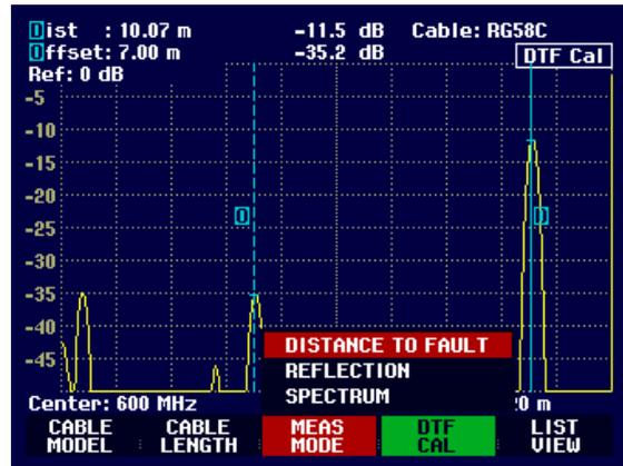
When SPECTRUM is selected, the R&S FSH3 turns off the tracking generator and displays the spectrum over the frequency range of the DTF measurement. To indicate that the R&S FSH3 is in the spectrum mode, **DTF Spectrum** is displayed in the top right-hand corner of the screen. Otherwise, the R&S FSH3 uses exactly the same settings as it did for DTF measurements.
