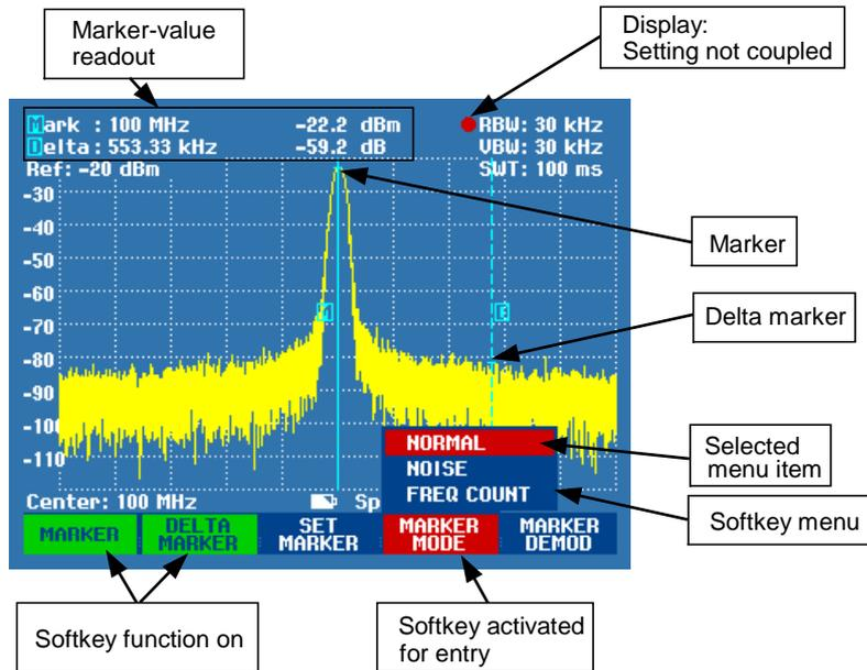
The colour of the softkey labelling and its background indicate the status of the softkey function in question:
