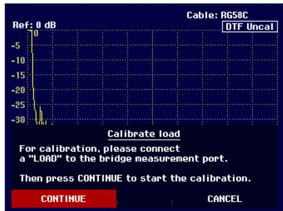
While LOAD calibration is in progress, the R&S FSH3 outputs the message "Calibrating LOAD, please wait...".
