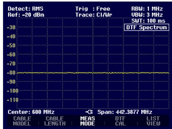
When REFLECTION is selected, the R&S FSH3 measures the return loss over the frequency range which has been selected for the distance-to-fault cable measurement. This means, for example, an antenna can be matched without altering the test setup. The R&S FSH3 automatically switches the VSWR Bridge R&S FSH-Z2 over to the VSWR measurement mode if REFLECTION has been selected.
