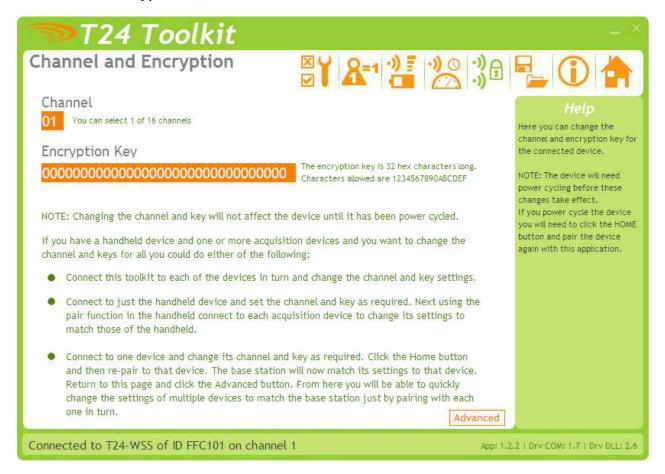
Here you can change the channel and encryption key for the acquisition module device.
