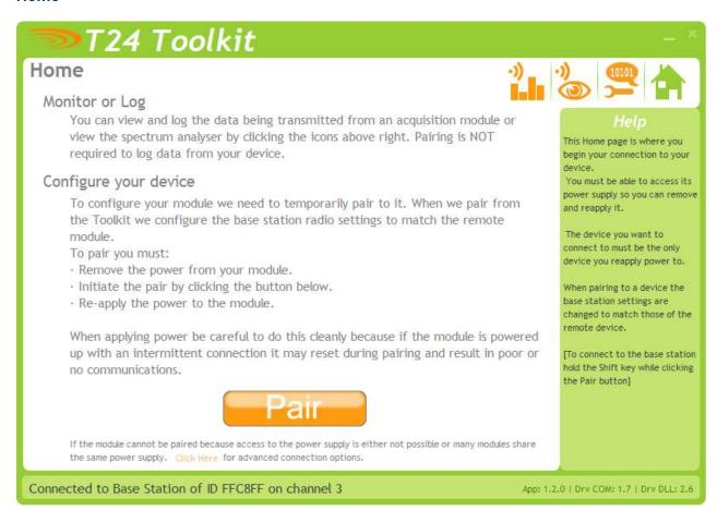
We now have successful communications with the base station so we can now pair with our device or we can select the Spectrum Analyser mode or Data Provider Monitor mode.
