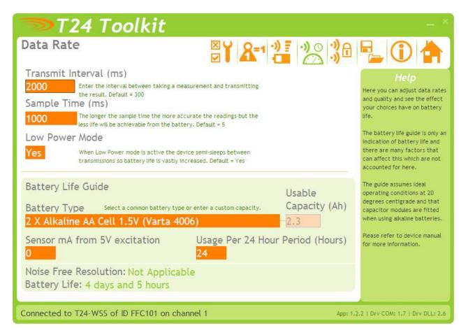
This page allows you to select the rate at which data is transmitted from the acquisition module and the quality. By selecting low power mode and entering some other information the toolkit will also give guides on achievable battery life.
