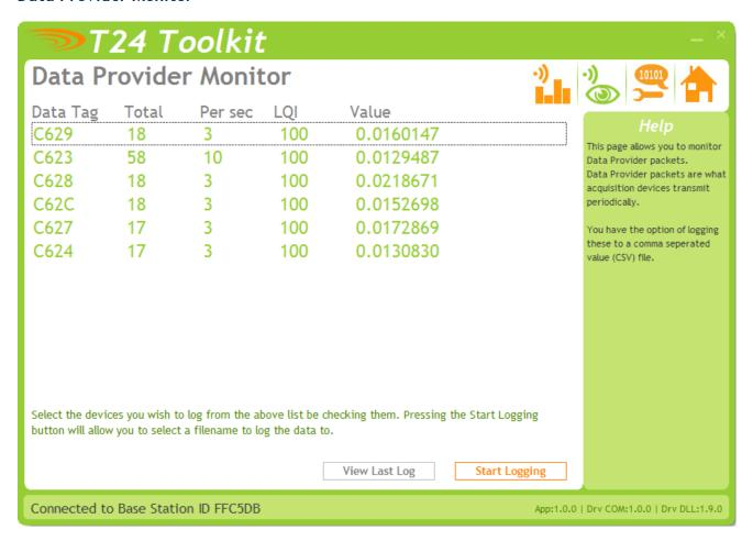
T24 acquisition devices normally operate in low power mode and periodically transmit Data Provider packets
