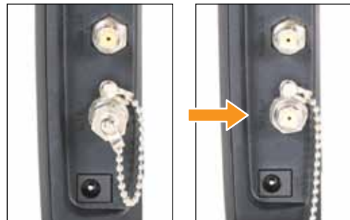
Remove Cap from "SAT Rcvr" on DCCK Device
