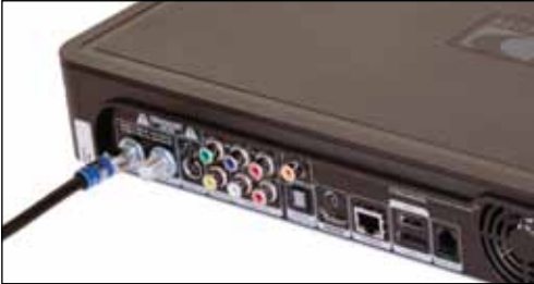
Disconnect Coaxial Cable from Receiver
