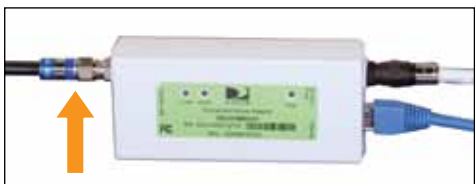
Disconnect Coaxial Cable from Connected Home Adapter
