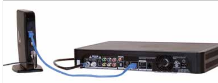
Connect Ethernet Cable to DIRECTV Receiver
