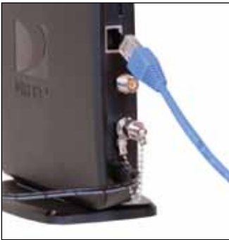
Connect Ethernet to DCCK Device
