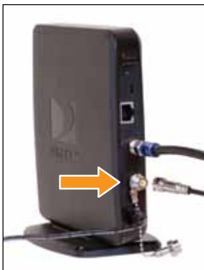
Connect Enclosed Coaxial Cable to "SAT Rcvr" on DCCK Device
