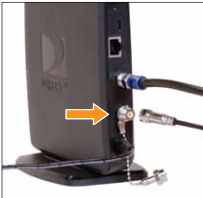
Connect Enclosed Coaxial Cable to "SAT Rcvr" on DCCK Device
