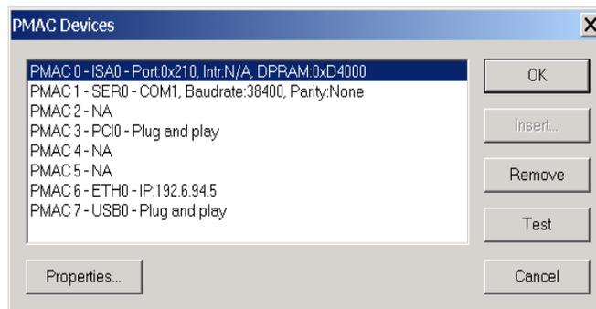
3. Once a PMAC is listed in the PMAC Select window, it is registered. After a device is registered, it should be tested. At this time, the following screen displays and the device is ready to use in any application.
