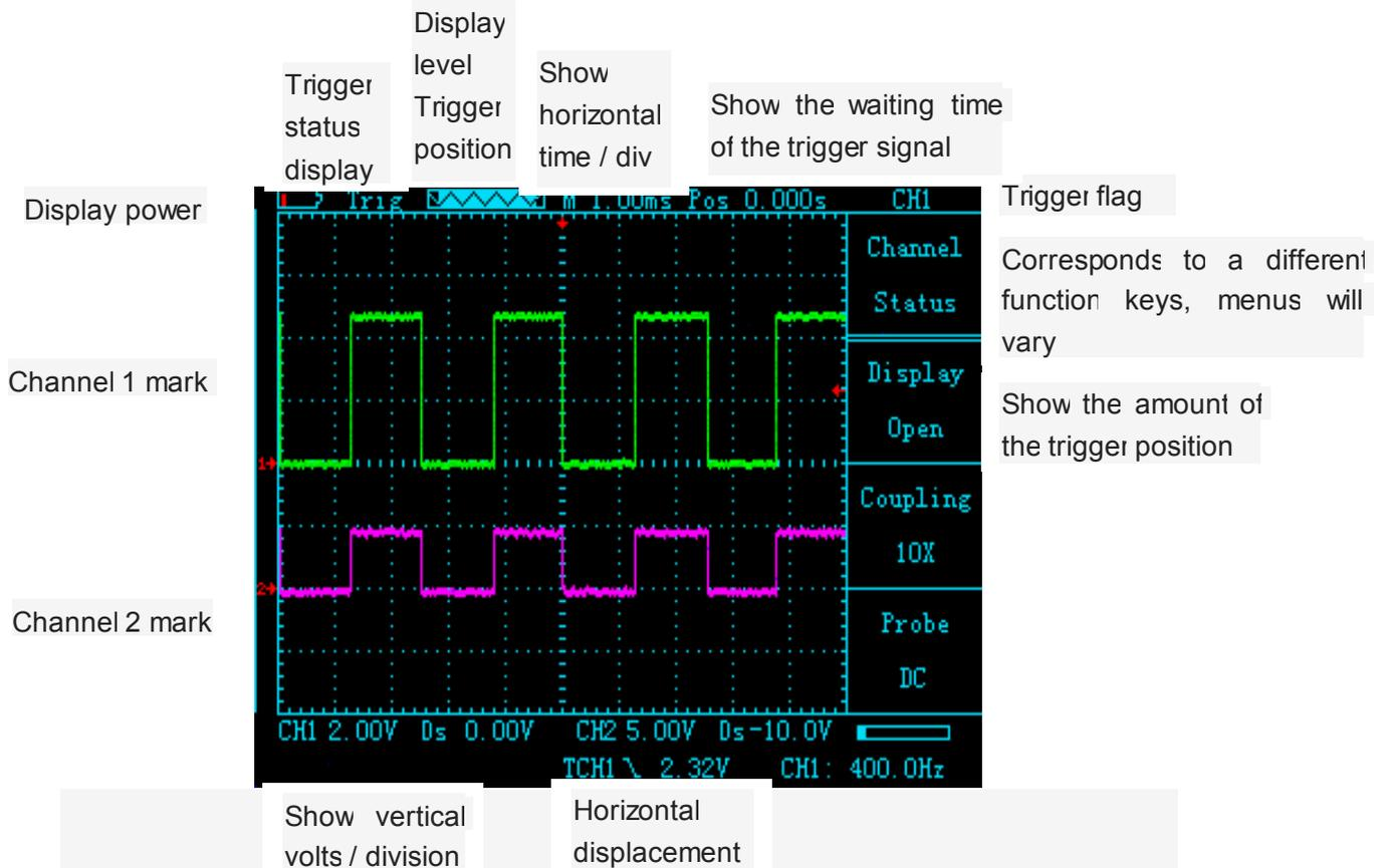
**Figure 1-3 Interface is shown in Figure**
