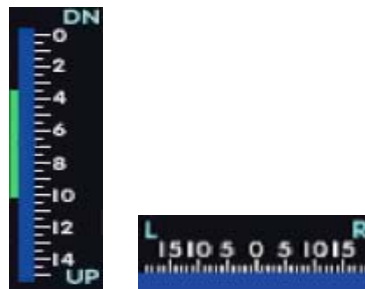
Figure 4.4: Stabilizer and rudder position displays, respectively
