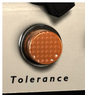
Figure 4: The Tolerance lamp indicates when a feedback is on its way, or when it is about to die.
