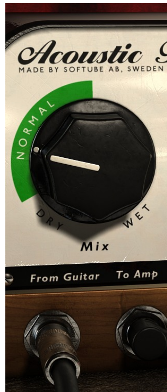
Figure 1: The Mix knob goes from dry (100% input signal) to wet (100% feedback effect). The normal setting is somewhere between 20 and 50 percent.
