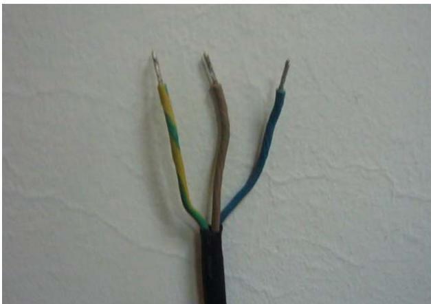
6. Respectively connect the Brown, Blue and Green/Yellow wires to the Line, Neutral and Ground terminals of an AC power source providing AC voltage of 100~277V.
