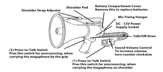
Megaphone for handheld or shoulder-slung use (straps supplied). Detachable anti-howl microphone with on-off switch and volume control. Metal and ABS construction.
