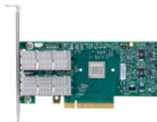
Figure 7: Mellanox MCX314A-BCBT, ConnectX-3 40GbE/FDR 56Gb/s InfiniBand Adapter
