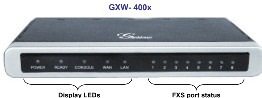
FIGURE 2: DIAGRAM OF GXW-400x DISPLAY PANEL
